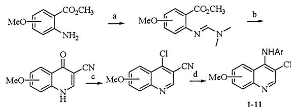
**Scheme 1.** (a) DMF-DMA, reflux; (b) LiCH<sub>2</sub>CN, THF, –78 °C, then HOAc, rt; (c) POCl<sub>3</sub>, reflux; (d) ArNH<sub>2</sub>, EtOCH<sub>2</sub>CH<sub>2</sub>OH, reflux.
