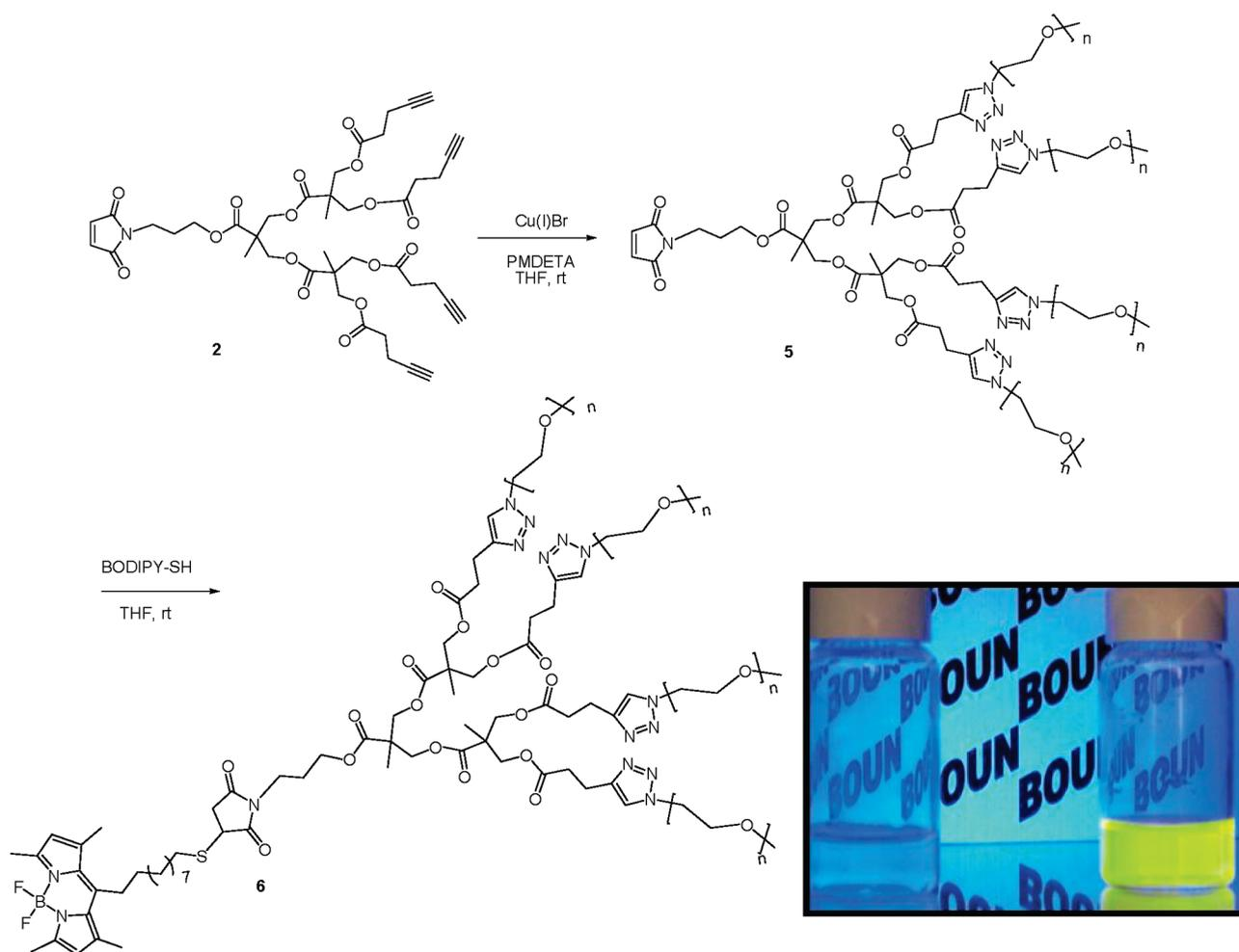
**Figure 4.** Orthogonal functionalization of dendron 2. Inset: Aqueous solution of BODIPY-SH (on the left) and aqueous solution of polymer conjugated BODIPY-SH 6 (on the right).
