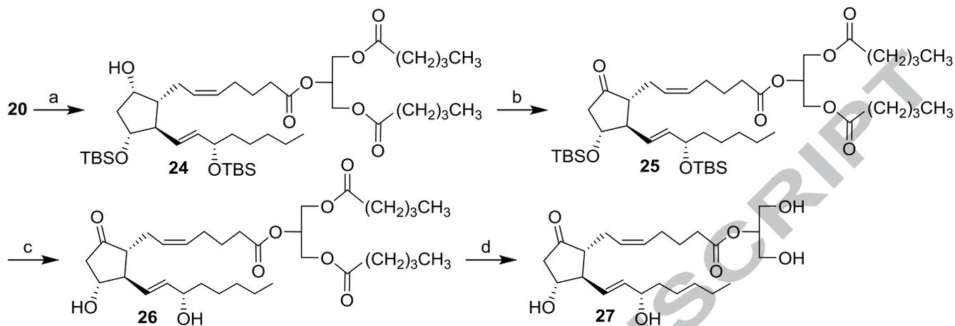
Reagents and conditions: (a) HO-CH[CH<sub>2</sub>-O-C(O)-(CH<sub>2</sub>)<sub>3</sub>CH<sub>3</sub>]<sub>2</sub>, carbonyldiimidazole, CH<sub>2</sub>Cl<sub>2</sub>, 0°C to r t, 24 h, 82%; (b) Dess-Martin periodinane, pyridine, CH<sub>2</sub>Cl<sub>2</sub>, 0°C to r t, 1 h, 97%; (c) 1% HCl, aqueous MeOH, r t, 5 min, 79%; (d) *Candida rugosa* lipase, EtOH, 2 h, 46%.
