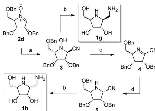
Scheme 3. Typical synthetic method for the preparation of new polyhydroxylated pyrrolidines **1g** and **1h** from cyclic nitron **2d**. Reagents and conditions: a) trimethylsilyl cyanide, MeOH, 50°C, 10 h; b) 1. Raney nickel,  $\text{H}_{2(g)}$ ,  $\text{Boc}_2\text{O}$ , MeOH, RT, 2 h; 2.  $\text{Pd}(\text{OH})_2$ ,  $\text{H}_{2(g)}$ , MeOH, RT, 10 h; 3. TFA, DCM, 0°C, 10 min; c)  $\text{MsCl}$ ,  $\text{Et}_3\text{N}$ , THF, 0°C, 1 min; d)  $\text{NaBH}_4$ , THF/MeOH (4:1), 0°C, 18 h.
