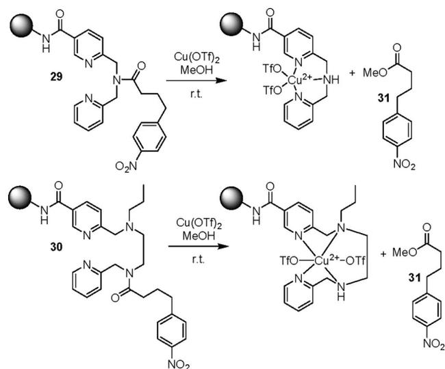
Scheme 8. Methanolysis reactions of an aliphatic amide bond with tetradentate construct **29** and tridentate construct **30**.
