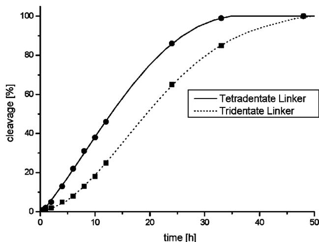
Figure 2. Kinetic data for the methanolysis of an aliphatic amide bond with tetradentate construct **29** and tridentate construct **30**.
