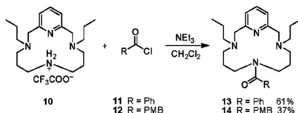
Scheme 3. Acylation of cyclic ligand **10** with carbonic acid chlorides **11** and **12**.
