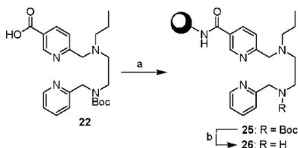
Scheme 6. Coupling of **22** to the solid support and cleavage of the Boc group. Reagents and conditions: (a) HypoGel400-NH<sub>2</sub>, DMF, 10 min, then **22** (1.3 equiv.), TBTU (1.3 equiv.), DIEA (8.0 equiv.), DMF, room temp., 8 h; (b)  $iPr_3SiH$  (3.0 equiv.), TFA/ $CH_2Cl_2$  (1:1), 2 h.
