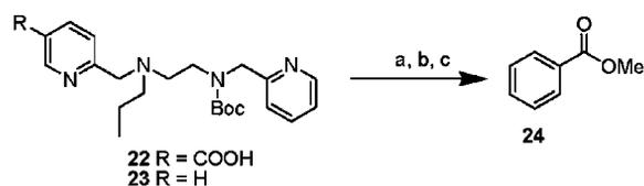
Scheme 5. Boc deprotection, coupling of benzoyl chloride, and subsequent methanolysis of tetradentate ligands **22** and **23**. Reagents and conditions: (a)  $iPr_3SiH$  (3.0 equiv.), TFA/ $CH_2Cl_2$  (1:1), 2 h; (b) benzoyl chloride (2.5 equiv.),  $NEt_3$  (2.5 equiv.),  $CH_2Cl_2$ , 0 °C  $\rightarrow$  room temp., 15 h; (c)  $Cu(OTf)_2$  (1.0 equiv.), MeOH, room temp., 15 h, 55%.
