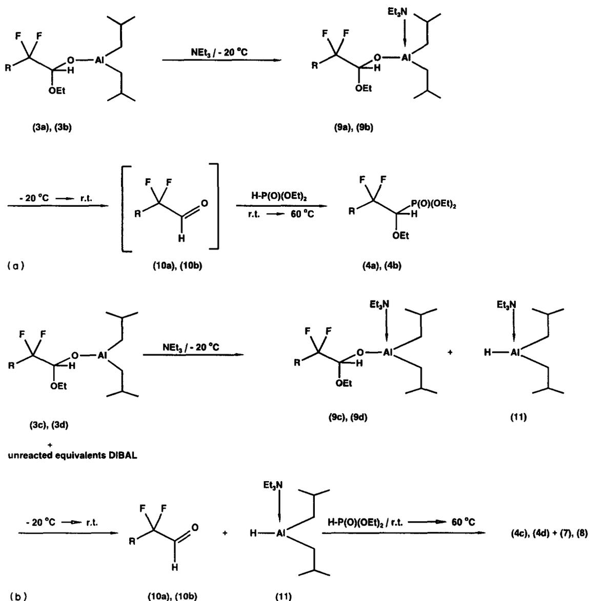
Scheme 3. The influence of triethylamine on the reduction process and on the reaction of compounds 3 with diethylphosphite. (a) 3a,4a,9a,10a, R = F; 3b,4b,9b,10b, R = CH<sub>3</sub>. (b) 3c,4c,7,9c,10c, R = Ph; 3d,4d,8,9d,10d, R = 3-CF<sub>3</sub>-Ph.
