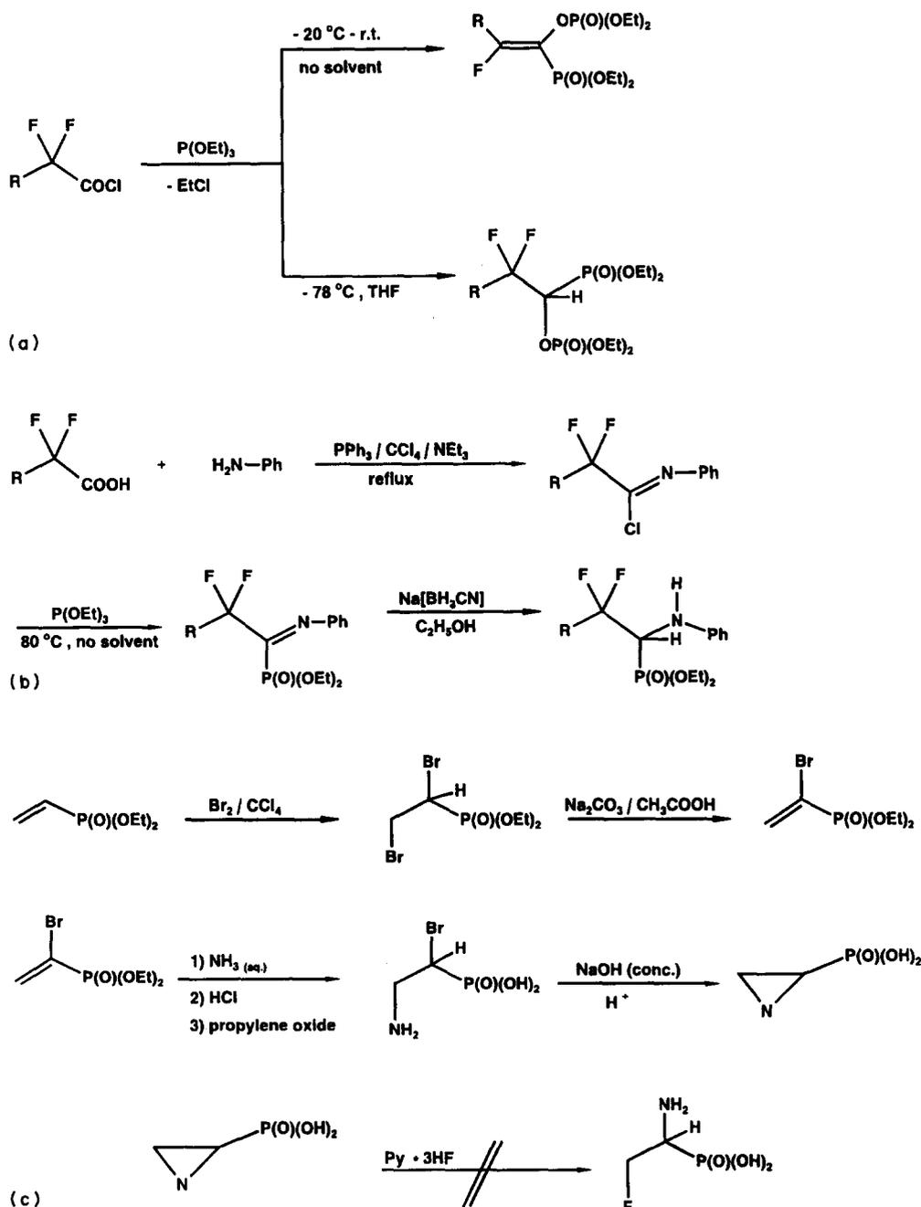
Fig. 1. (a) Reaction of 2-(4-fluorophenyl)-2,2-difluoroacetyl chloride with triethylphosphite [8,9] ( $\text{R} = 4\text{-F-Ph}$ ); (b) trifluoroacetimidoyl chlorides as intermediates in the aminophosphonic acid synthesis ( $\text{R} = \text{F}$ ); and (c) aziridines as potential precursors to  $\beta$ -fluorinated  $\alpha$ -aminophosphonic acids.
