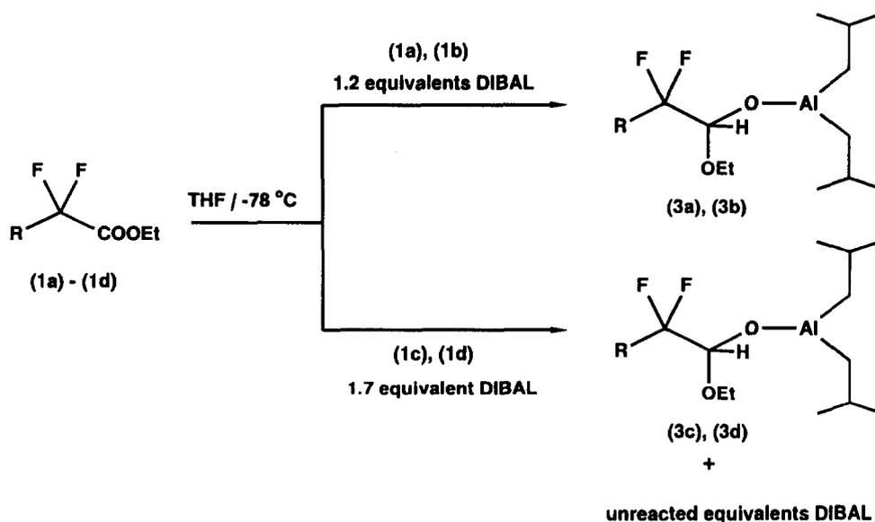
Scheme 1. Different reduction conditions for aliphatic compounds **1a–d**: **1a,3a**, R = F; **1b,3b**, R = CH<sub>3</sub>; **1c,3c**, R = Ph; **1d,3d**, R = 3-CF<sub>3</sub>-Ph.
