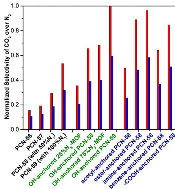
**Figure 5.** Normalized CO<sub>2</sub> adsorption selectivity over N<sub>2</sub> (obtained from CO<sub>2</sub> sorption amount (1 atm and 273 K for red bars; 1 atm and 296 K for blue bars) divided by N<sub>2</sub> sorption amount at 1 atm and 77 K) for three sets of samples (Zr-MOFs with various loadings of azide group, black marks; hydroxyl group anchored onto Zr-MOFs with various loadings of azide group, green marks; and diverse functional group anchored onto PCN-58, blue marks).
