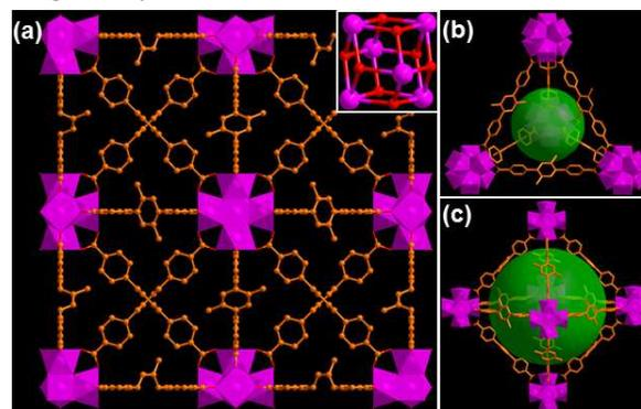
**Figure 1.** (a) View of the structure of PCN-56 as a representative, bearing two methyl groups in each TPDC-derived linker. Accordingly, four methyl, two methyl azide, and four methyl azide groups are involved in each organic linker, respectively for PCN-57, PCN-58 and PCN-59. Inset: the  $Zr_6$  cluster. (b) Tetrahedral and (c) octahedral cages comprised  $Zr_6$  clusters and organic linkers in PCN-56. The cavities are highlighted with green spheres.
