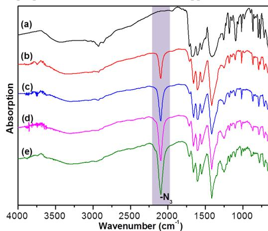
**Figure 4.** IR spectra of Zr-MOFs with (a) 0% N<sub>3</sub> (PCN-56), (b) 25% N<sub>3</sub>, (c) 50% N<sub>3</sub> (PCN-58), (d) 75% N<sub>3</sub>, and (e) 100% N<sub>3</sub> (PCN-59). The characteristic IR band (highlighted with light purple background) for azide group is at ~2100 cm<sup>-1</sup>. The intensity of this band is proportional to the azide loading of each MOF.
