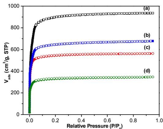
**Figure 2.** N<sub>2</sub> sorption properties for (a) PCN-56, (b) PCN-57, (c) PCN-58, and (d) PCN-59 at 77 K and 1 atm. Solid circles or squares: adsorption; open: desorption. The BET surface areas are 3741, 2572, 2185 and 1279 m<sup>2</sup>/g, respectively for PCN-56 to -59, which are comparable to calculated values (3317, 2416, 2131 and 1168 m<sup>2</sup>/g, respectively for PCN-56 to -59).
