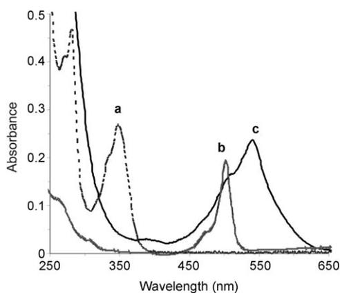
Figure 5. UV/Vis spectra of a) pyrene macrocycle **28** ( $1 \times 10^{-6}$  M; multiplied by 10), b) BODIPY macrocycle **31** ( $5 \times 10^{-6}$  M), and c) FBMH **33** ( $1.6 \times 10^{-5}$  M) in  $\text{CH}_2\text{Cl}_2$ .
