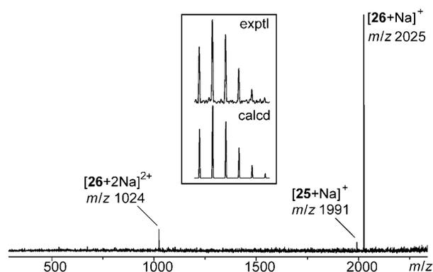
Figure 4. ESI-FTICR mass spectrum of the raw product obtained from the reaction of **25** with  $\text{Na}_2\text{S} \cdot (\text{H}_2\text{O})_x$  yielding thiophene-centered **26**.
