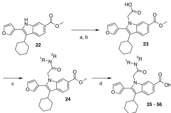
Scheme 1. Synthesis of *N*-acetamidindole NS5B inhibitors. Reagents and conditions: (a) NaH (1.25 equiv), DMF, 0 °C, 1 h then *tert*-butylbromoacetate (1.24 equiv), rt, 18 h (86% yield); (b) TFA, 4 h, rt (99% yield); (c) TBTU or HATU (1.2 equiv), Et<sub>3</sub>N (5 equiv), DMF or DMSO, rt, 10 min then <sup>1</sup>R<sup>2</sup>RNH, rt, 1–18 h; (d) 10 N NaOH (5–10 equiv), 5:1 DMSO-water, 1–2 h, then purification by reversed-phase HPLC (>95% homogeneity).
