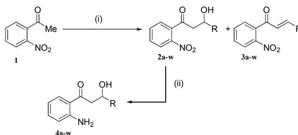
Scheme 1. Reagents and conditions: (i) RCHO (1.1 equiv), LDA (2.5 equiv), THF, -78 °C, 1 h, 48-69% (ii) 10% Pd/C (20% wt), EtOH, 50 psi, 1 h, 78-91%
