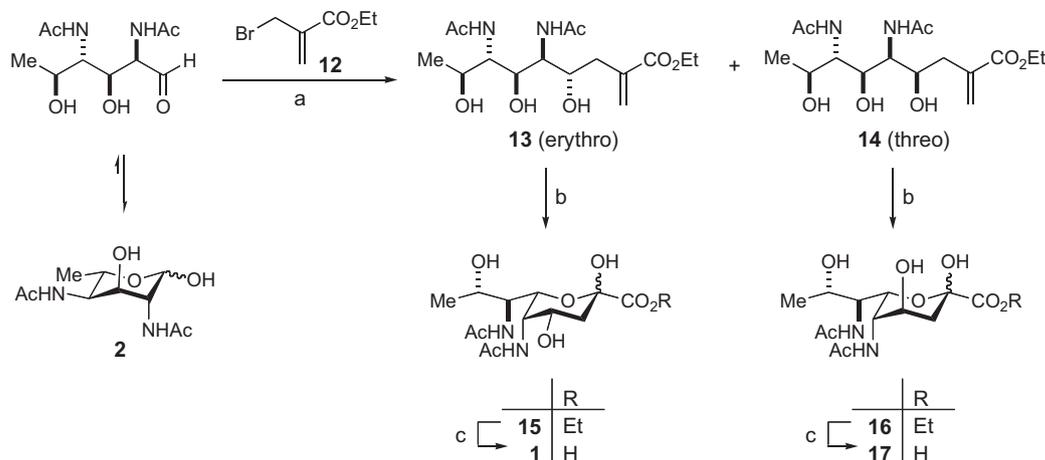
**Scheme 4.** Reagents and conditions: (a) In, 0.1 N HCl–EtOH (1:6), 40 °C, 12 h, 77%, **13/14** = 5:4; (b) O<sub>3</sub>, MeOH, –78 °C, 30 min, then 30% H<sub>2</sub>O<sub>2</sub>, H<sub>2</sub>O, HCO<sub>2</sub>H, 90 min, for **15**: 85%,  $\alpha/\beta$  = 5:1; for **16**: 86%,  $\alpha/\beta$  = 3:1; (c) TEA–H<sub>2</sub>O (1:3), 0 °C, 2 h, for **1**: 96%, for **17**: 92%.
