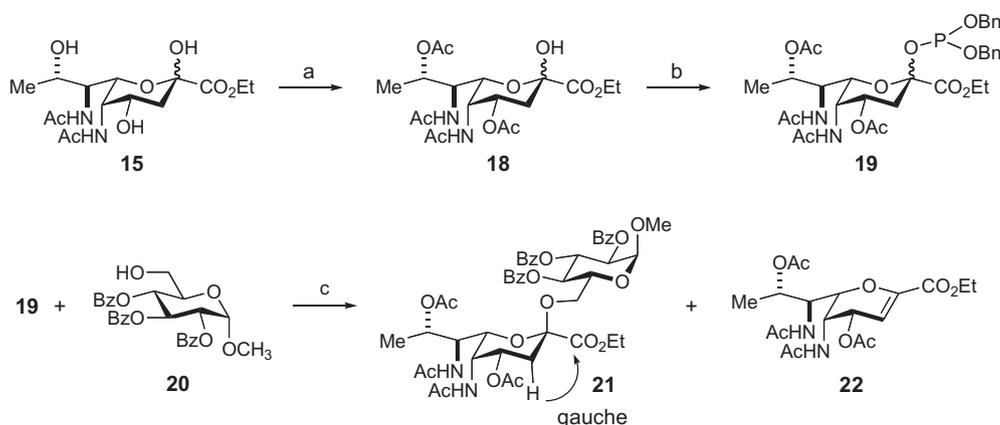
**Scheme 5.** Reagents and conditions: (a) Ac<sub>2</sub>O, pyridine, 0 °C, 12 h, 73%,  $\alpha/\beta$  = 8:1; (b) Et<sub>2</sub>NP(OBn)<sub>2</sub>, 1H-tetrazole, THF, 2 h, 94%; (c) TMSOTf, CH<sub>3</sub>CN, 0 °C, 3 h [**21**: 28% ( $\alpha/\beta$  = 10:1), **22**: 47%] or CH<sub>2</sub>Cl<sub>2</sub>, rt, 6 h [**21**: 35% ( $\alpha$  only), **22**: 62%].
