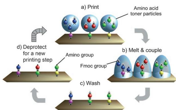
**Figure 1.** Particle-based Merrifield synthesis. a) A laser printer delivers Fmoc amino acid–OPfp esters embedded within toner particles to specific locations on a solid support, on which b) the particles are melted after transfer. Melting enables the amino acid derivatives to diffuse and undergo coupling to the support. A synthetic cycle is completed when c) excess monomers are washed away, and d) the Fmoc protecting group is removed. Repeated coupling cycles generate a peptide array.
