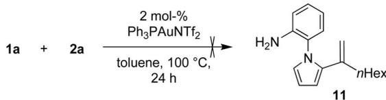
Scheme 3. Reaction between **1a** and **2a** under standard conditions.
