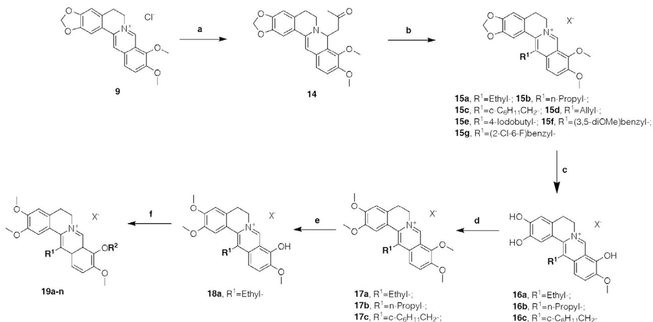
**Scheme 2.** Synthesis of 5,6-dihydrodibenzo[*a,g*]quinolizinium derivatives of P2X<sub>7</sub> antagonist. Reagents and conditions: (a) acetone, aq 45% NaOH, H<sub>2</sub>O, rt, 90%; (b) substituted alkyl halide or benzyl halide, acetonitrile or toluene, reflux, 47–54%; (c) i-AlCl<sub>3</sub>, toluene, reflux; ii–0.8–1.2 N HCl, reflux, 96%; (d) dimethyl sulfate or methyl iodide, aq 50% NaOH, 81%; (e) LiCl, DMF, 140 °C, 90%; (f) R<sup>2</sup>X, NaI, acetonitrile, reflux, 60–80%.
