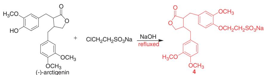
Figure 2. Synthetic route for alkylation derivative of 4.
