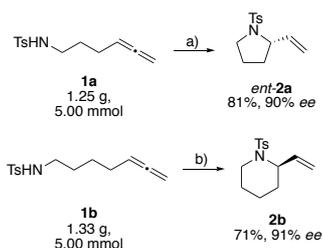
**Scheme 4.** Gram-scale catalysis. Reagents and conditions: a)  $[\{\text{Rh}(\text{cod})\text{Cl}\}_2]$  (2.0 mol%), *ent*-**L5** (5.0 mol%), TFA (10 mol%),  $\text{CH}_2\text{Cl}_2$  (0.2 M), 60 °C, 18 h; 81%, 90% ee. b)  $[\{\text{Rh}(\text{cod})\text{Cl}\}_2]$  (2.0 mol%), **L5** (5.0 mol%), PPTS (10 mol%), DCE (0.2 M), 80 °C, 18 h; 71%, 91% ee.
