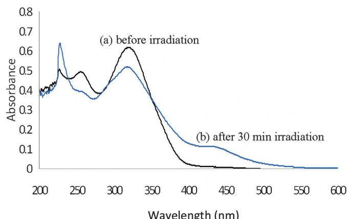
**Fig. 11.** Recovery of the trans  $\pi-\pi^*$  band at maximum absorbance 319 nm of complex **7** on heating at a rate of  $2\text{ }^\circ\text{C min}^{-1}$ .
