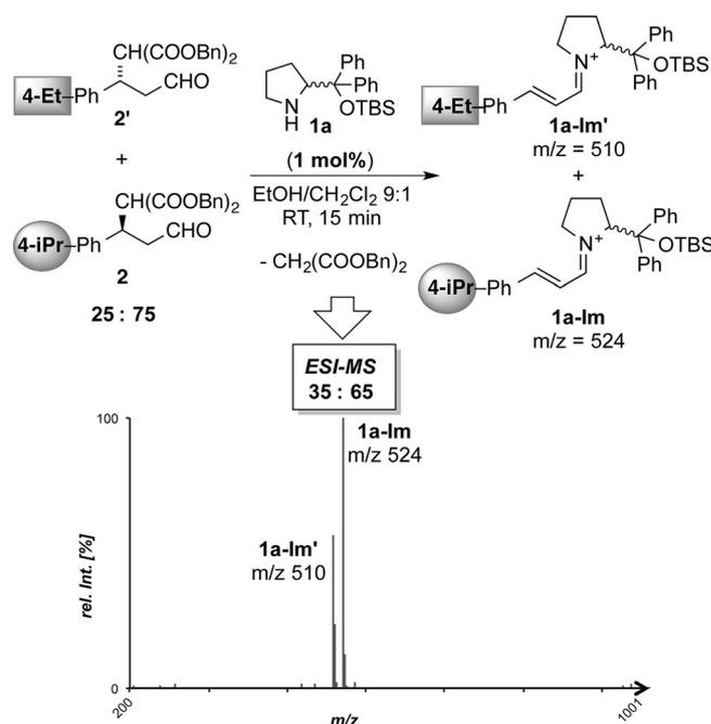
**Figure 5.** ESI-MS back reaction screening with 1 mol% of racemic catalyst **1a**. Below, typical ESI-MS spectra obtained under screening conditions.
