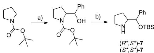
**Scheme 3.** Synthesis of racemic catalysts **7**. Conditions: a) *sec*-BuLi, TMEDA, Et<sub>2</sub>O,  $-78^{\circ}\text{C}$ ; then benzaldehyde,  $-78^{\circ}\text{C}$  to r.t., separation of diastereoisomers by FC. b) (1) AcOH/3M HCl, r.t. (2) TBSOTf, NEt<sub>3</sub>, CH<sub>2</sub>Cl<sub>2</sub>,  $0^{\circ}\text{C}$  to r.t.
