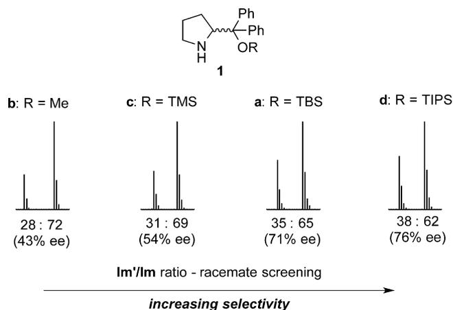
**Figure 6.** **Im'/Im** ratios monitored by ESI-MS. In brackets: enantioselectivity of catalysts **1a-d** calculated from eq. (1).
