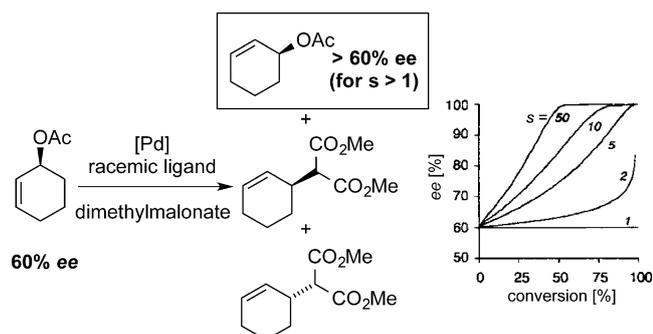
**Figure 1.** Evaluation of a racemic catalyst based on the concept of Lloyd-Jones.<sup>[4]</sup> The diagram shows the theoretical curves for the increase of *ee* with conversion calculated for different selectivity factors (*s*) starting from scalemic acetate with 60% *ee*.
