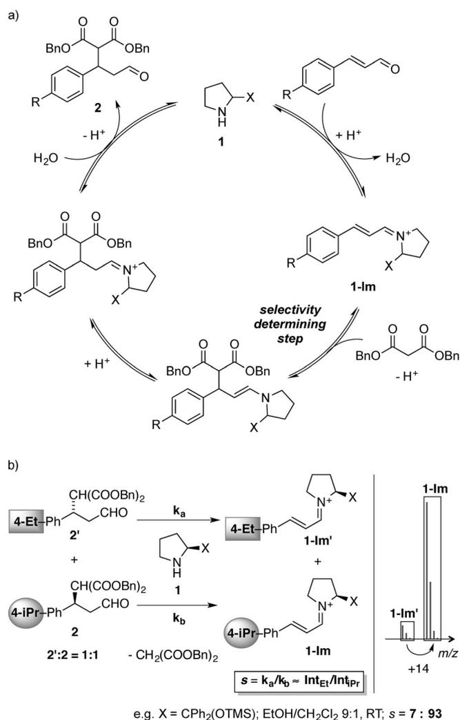
**Figure 3.** a) Simplified mechanism of the amine-catalyzed Michael addition. b) ESI-MS screening with enantiopure catalysts.
