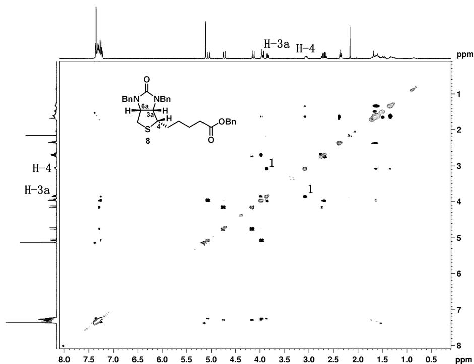
Figure 3. 2D NOESY spectrum of **8**. Note: peak **1** in the figure is the cross peak between H-3a ( $\delta$  3.84 ppm) and H-4 ( $\delta$  3.03–3.06 ppm).
