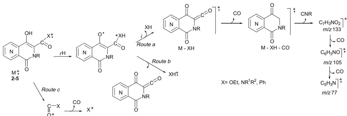
Scheme 3. Mass spectra fragmentation pathways of naphthyridinones **2–5** under EI conditions.
