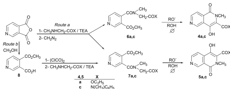
**Scheme 2.** Synthesis of *N*-lactam substituted naphthyridinones **4** and **5**.
