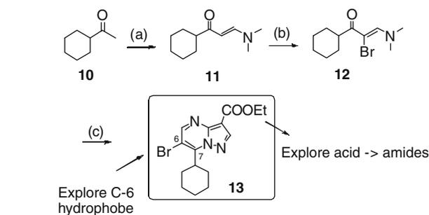
**Scheme 2.** Synthesis of advanced intermediate **13**. Reagents and conditions: (a) Brederick's reagent (*t*-butoxybis(dimethylamino) methane),  $60^\circ\text{C}$ ,  $93\%$ ; (b) bromine, DCM, triethylamine,  $0^\circ\text{C}$  to rt; (c) 5-amino-1*H*-pyrazole-4-carboxylate, ethanol,  $30\%$  hydrogen bromide in acetic acid, reflux,  $27\%$  (steps (b) and (c)).
