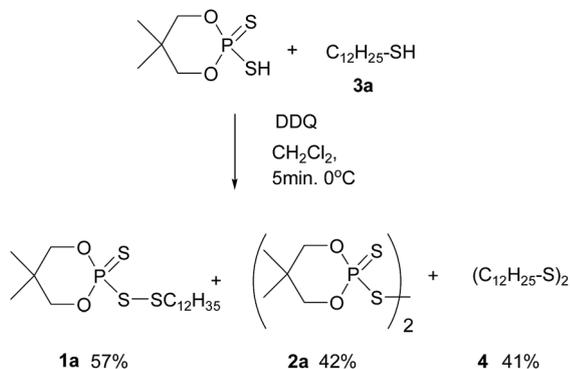
Fig. 2 Oxidation of phosphorodithioic acid and thiol **3a** mixture by DDQ.
