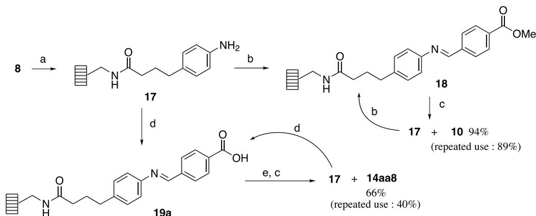
**Scheme 4.** Model synthesis of azomethines on a solid support using an aniline linker **17**. Reaction conditions: (a) 4-(4-*tert*-butoxycarbonylamino)phenylbutyric acid, DIC, HOBt, DCM, then TFA, DCM; (b) methyl 4-formylbenzoate, DMF, rt, 24 h; (c) 4-octyloxyaniline, 50 °C, 3 h; (d) 4-formylbenzoic acid, DMF, rt, 24 h; (e) 1-nonanol, DIC, DMAP, DCM, rt, 3 h.
