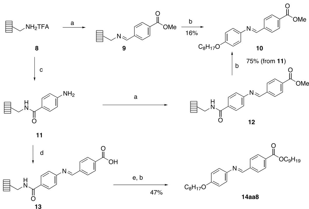
**Scheme 2.** Model synthesis of azomethines on a solid support from **8** or **11**. Reaction conditions: (a) methyl 4-formylbenzoate, DMF, rt, 24 h; (b) 4-octyloxyaniline, 50 °C, 3 h; (c) 4-*tert*-butoxycarbonylaminobenzoic acid, DIC, HOBT, DCM, then TFA, DCM; (d) 4-formylbenzoic acid, DMF, rt, 24 h; (e) 1-nonanol, DIC, DMAP, DCM, rt, 3 h.
