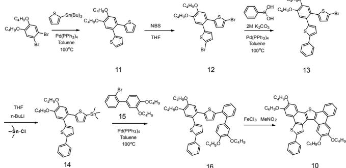
**Scheme 5.** Retrosynthesis of compound **10** for identification of its chemical structure.
