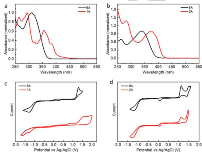
**Figure 3.** (a, b) UV-vis absorption spectra of **6A/1A** and **8A/2A**; (c, d) cyclic voltammograms of **6A/1A** and **8A/2A** in dry dichloromethane.
