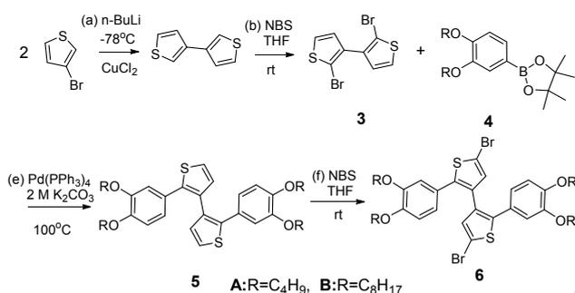
Scheme 1. Synthesis of the key intermediate of **6**.
