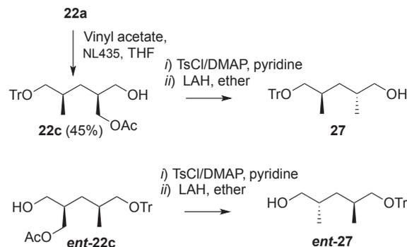
**Scheme 4.** Preparation of *anti* stereodiad alcohols **27/ent-27**.
