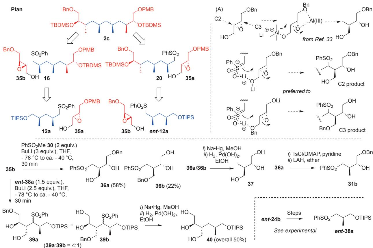
**Scheme 7.** Alternate plan and model experiments with epoxide **35b**.
