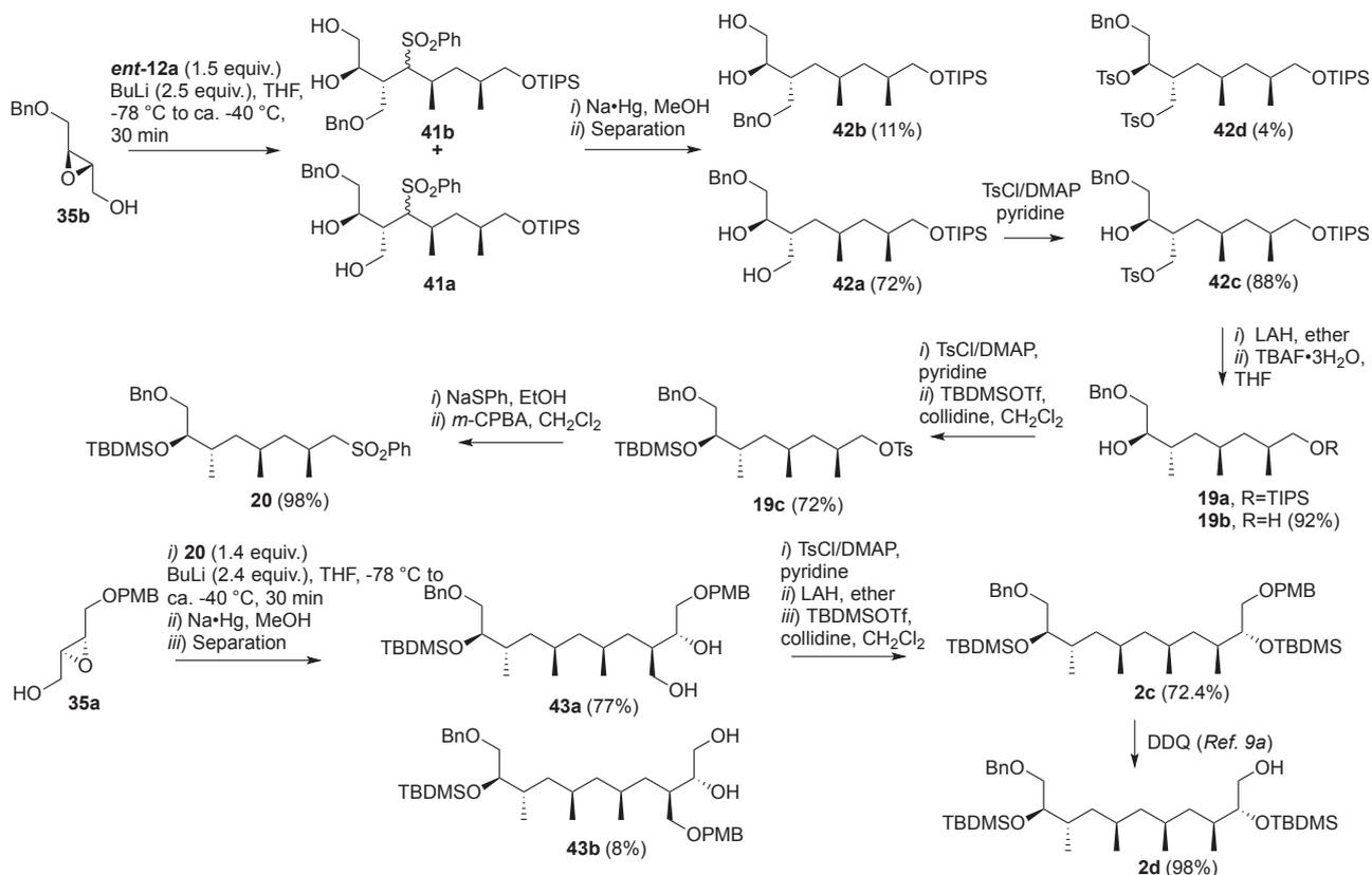
**Scheme 8.** Synthesis of the Morcken's intermediates **2c/2d** from sulfone **ent-12a**.
