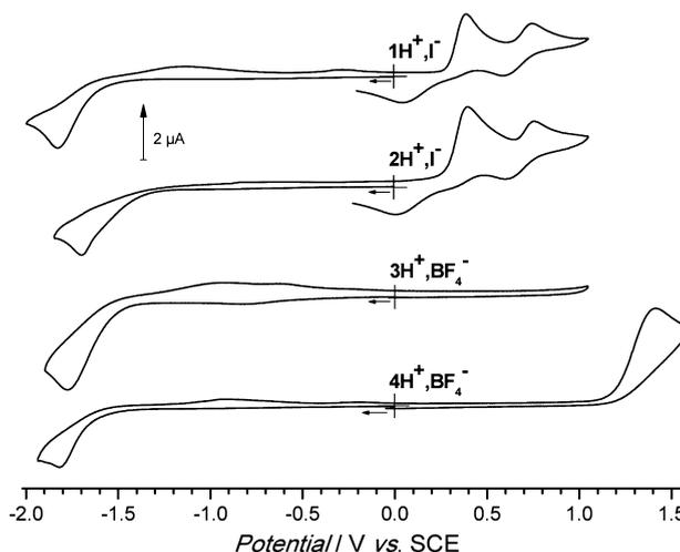
**Figure 2.** CVs of imidazolium salts in DMF containing 0.1 M TBAPF<sub>6</sub> (under Ar, WE: Pt, Ø = 1 mm, ν = 0.1 V s<sup>-1</sup>, c = 2.0 × 10<sup>-3</sup> M).
