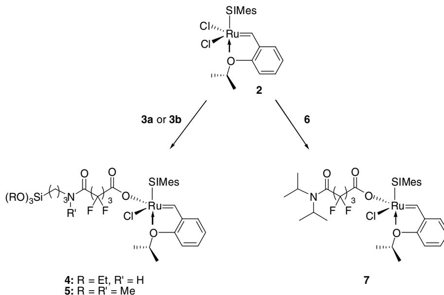
Scheme 2. Synthesis of the homogeneous, monocarboxylated ruthenium catalysts **4**, **5** and **7**.Table 1
