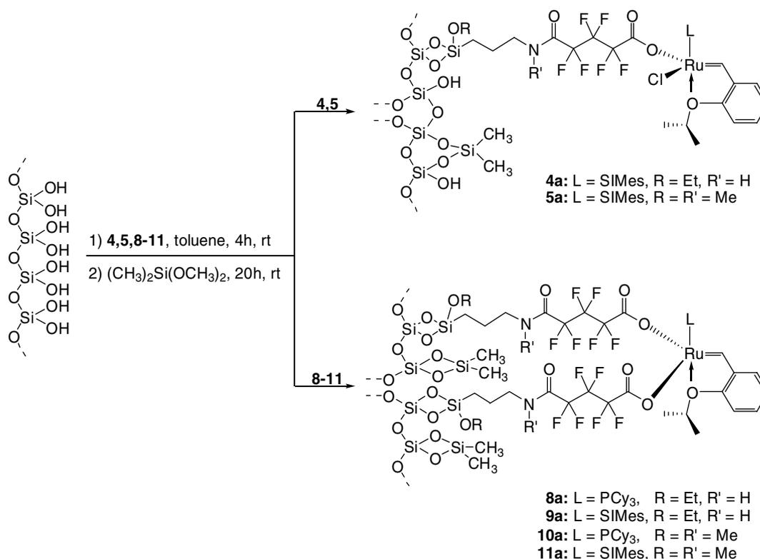
Scheme 4. Immobilization of the complexes **4, 5** and **8–11** onto silica gel.
