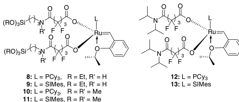
Scheme 3. Homogeneous, chlorine-free, disubstituted ruthenium catalysts **8–13**.
