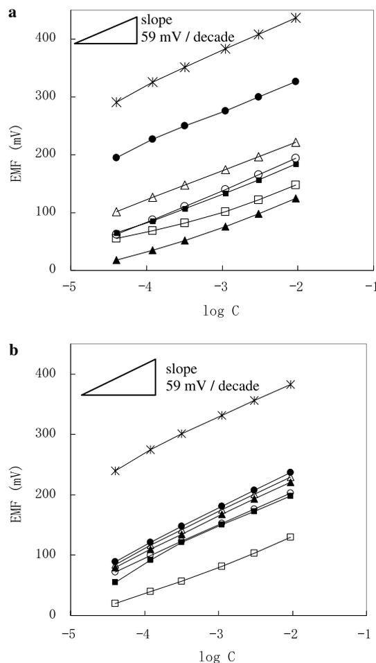
**Figure 2.** Membrane potential (electromotive forces; EMF) vs concentration curves for dopamine (●, DA), noradrenaline (■, NA), adrenaline (▲, AD), 2-phenylethylamine (\*, PEA), and inorganic cations (□,  $\text{Na}^+$ ; △,  $\text{K}^+$ ; ○,  $\text{NH}_4^+$ ), measured at room temperature with (a) membrane III incorporated with host **3** and (b) blank membrane without a host.
