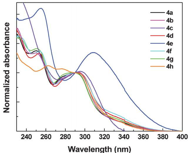
Fig. 2 Normalized absorption spectra of **4a–h** in dichloromethane (normalized at 290 nm).
