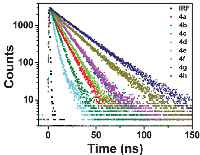
Fig. 4 Fluorescence decays of the synthesized compounds in dichloromethane. The samples are indicated in the legends. The sharp profile in black represents the instrumental response function (IRF).
