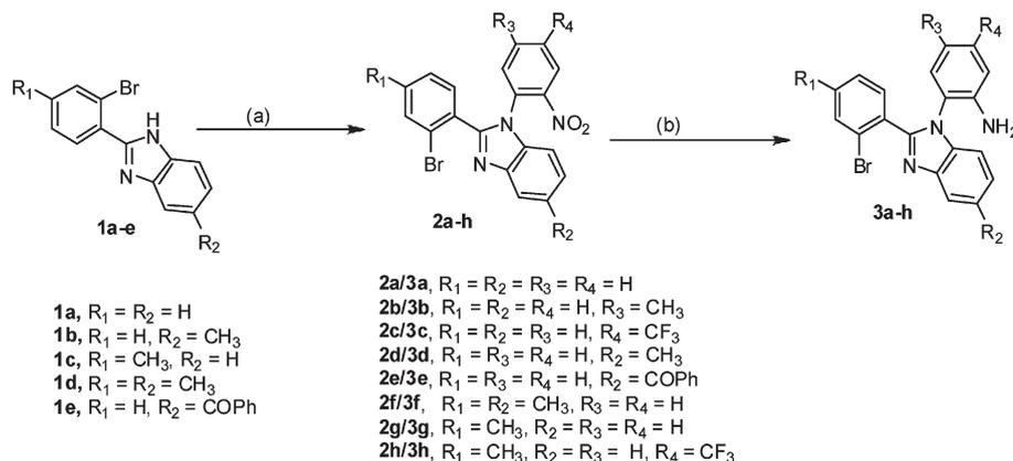
**Scheme 1** Synthesis of benzimidazole fused aromatic amines. Reagents and conditions: (a) acetone, KOH, *o*-fluoronitrobenzenes, reflux, 5 h. (b) Fe, AcOH, 80 °C, 1 h.
