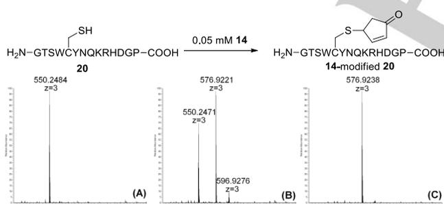
**Figure 1.** Mass spectrum of peptide (5  $\mu$ M) modified by **14** (50  $\mu$ M) in PBS buffer (pH = 7.4) at room temperature. The reaction was monitored by LCMS. (A) t = 0 min; (B) t = 2 min; (C) t = 12 min.
