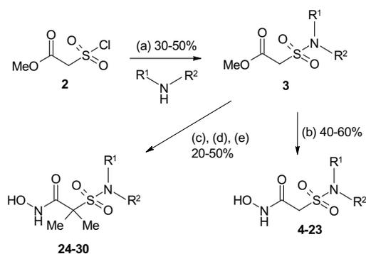
Scheme 1. Reagents and conditions: (a) DBU,  $\text{CH}_2\text{Cl}_2$ , 0 °C to rt; (b)  $\text{HONH}_2\cdot\text{HCl}$ ,  $\text{K}_2\text{CO}_3$ , MeOH, reflux; (c) MeI,  $\text{K}_2\text{CO}_3$ , DMSO, rt; (d) NaOH, MeOH,  $\text{H}_2\text{O}$ , reflux; (e) HATU, *N*-ethyl-diisopropylamine,  $\text{HONH}_2\cdot\text{HCl}$ , NMP, rt.
