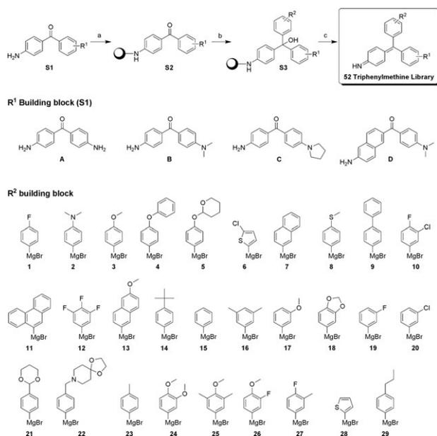
**Scheme 1** Synthesis of triphenylmethine library. *Reagents and conditions:* (a) 2-chlorotrityl chloride resin ( $1.37 \text{ mmol g}^{-1}$ ), pyridine,  $\text{CH}_2\text{Cl}_2$ -DMF; (b) Grignard reagents, THF,  $62^\circ\text{C}$ ; (c) 1% TFA,  $\text{CH}_2\text{Cl}_2$ .
