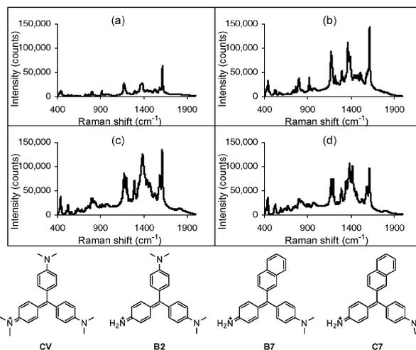
**Fig. 3** SERS spectra of PEG encapsulated nanotags and structure of TM compounds: (a) **CV**, (b) **B2**, (c) **B7**, and (d) **C7**.
