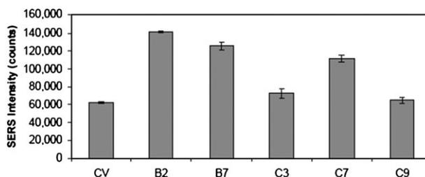
**Fig. 2** SERS intensities of PEG encapsulated nanotags. The average intensities of five individual measurements with error bars denoting their standard deviation. SERS spectra were obtained from excitation at 633 nm with laser power of 3 mW.
