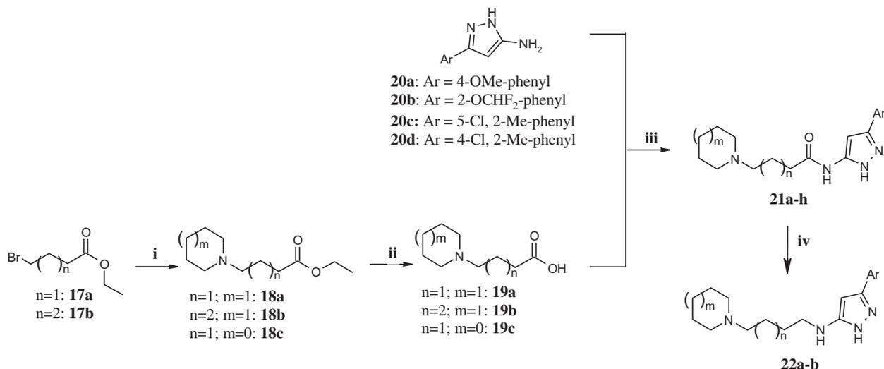
**Scheme 4.** Route C reagents and conditions: (i) piperidine, toluene, reflux; (ii) NaOH, water, reflux; (iii) CDI, 1,2-dichloroethane, 50 °C; (iv) LiAlH<sub>4</sub>, THF reflux.
