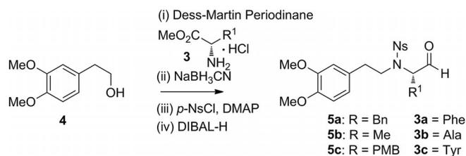
Scheme 2. Synthesis of  $\alpha$ -chiral aldehydes **5a–5c**: (i) CH<sub>2</sub>Cl<sub>2</sub>, 15 min, room temp.; (ii) MeOH, 12 h, room temp.; (iii) py, 3 h, room temp.; (iv) CH<sub>2</sub>Cl<sub>2</sub>, 2 h, –78 °C.
