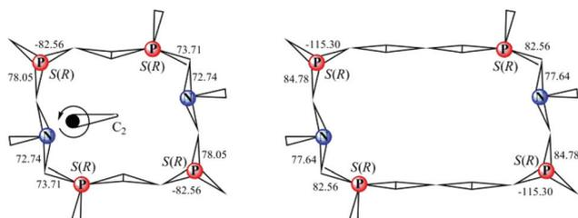
Fig. 3 Dale's wedge representation of the [77] and [99] conformations of the 14- and 18-membered macrocyclic aminomethylphosphines (angles are given in degrees, °).
