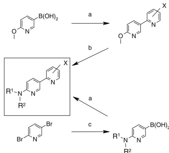
**Scheme 5.** (a) ArX, Pd(PPh<sub>3</sub>)<sub>4</sub>, 2 N Na<sub>2</sub>CO<sub>3</sub>, DMF, 80 °C, 35–70%; (b) (i) POCl<sub>3</sub>, DMF, 53–85%, (ii) R<sup>1</sup>R<sup>2</sup>NH, NMP, microwave, 250 °C, 7–77%; (c) (i) R<sup>1</sup>NHR<sup>2</sup>, pyridine, reflux, 96%, (ii) *n*BuLi, B(O<sup>*i*</sup>Pr)<sub>3</sub>, Et<sub>2</sub>O, 48–61%.
