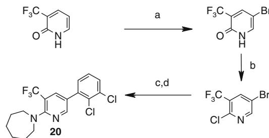
**Scheme 4.** (a) Br<sub>2</sub>, MeOH; (b) PhPOCl<sub>2</sub>, 75%; (c) homopiperidine, THF, 94%; (d) Pd(PPh<sub>3</sub>)<sub>4</sub>, 2 N Na<sub>2</sub>CO<sub>3</sub>, DME, 80 °C, 70%.
