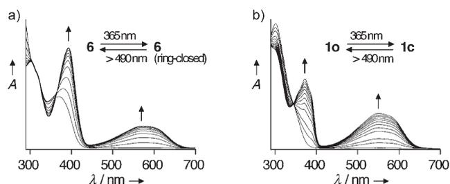
**Figure 1.** Changes in the UV/Vis absorption spectra of compound **6** (a) and **1o** (b) upon irradiation with  $\lambda = 365\text{ nm}$  (benzene solutions,  $2.65 \times 10^{-5}\text{ M}$  and  $8.22 \times 10^{-5}\text{ M}$  for **6** and **1o**, respectively). Spectra were recorded every 10 seconds until a 90-second period (for **6**) and a 120-second period (for **1o**) were completed.
