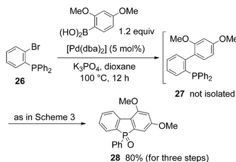
**Scheme 5.** Synthesis of phosphole **28** from **26**. dba = dibenzylideneacetone.
