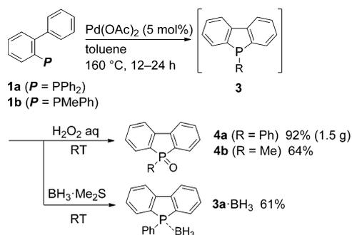
**Scheme 3.** Palladium-catalyzed synthesis of phosphole.
