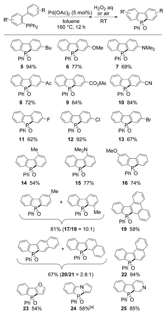
**Scheme 4.** Reaction scope. Reaction conditions: biarylphosphine (0.30 mmol), Pd(OAc)<sub>2</sub> (0.015 mmol), and toluene (1.0 mL) in a sealed tube at 160 °C, for 12 h. Yields of isolated products are shown. [a] The reaction was set up in a glovebox because of the sensitivity of the starting phosphine to oxygen.
