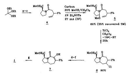
*Reagents:* a) cinnamyl alcohol, cat. propionic acid, reflux, 4h. b) KOH, MeOH, reflux, 6h, 82% over two steps. c) i.  $(COCl)_2$ , cat. DMF, PhCH<sub>3</sub>, ii. (S)-(+)-2-(methoxymethyl)pyrrolidine, 76%. d) H<sub>2</sub>, 5% Pd/C, NaOMe, MeOH, 88%. e) i. LDA, THF, -50 to -40°C, ii. (+)-(2R,8aS)-(camphorsulfonyl)oxaziridine (Davis' reagent), 78%. f) i. NCS, DMS, CH<sub>2</sub>Cl<sub>2</sub>, -30 to -20°C ii. Et<sub>3</sub>N, 76%. g) NH<sub>3</sub>, MeOH, 69%.
