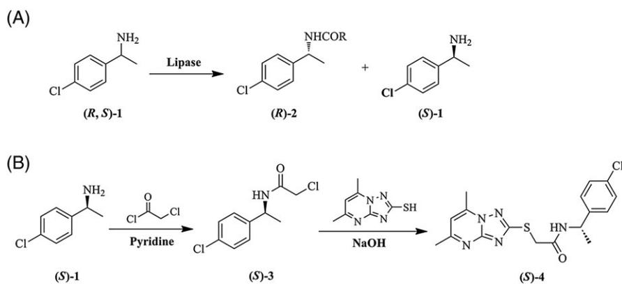
**SCHEME 1** A, The lipase-catalyzed resolution of (R,S)-1-(4-chlorophenyl) ethylamine ((R,S)-1). B, The synthesis of (S)-*N*-(1-(4-chlorophenyl)ethyl)-2-(5,7-dimethyl-[1,2,4]triazolo[1,5-*a*]pyrimidin-2-ylthio)acetamide ((S)-4).
