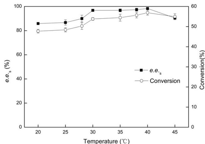
**FIGURE 3** The effects of temperature on the enantioselective amidation of (R,S)-1. The reactions were carried out at 200 rpm at different temperatures for 24 hours; the experiment used 100  $\mu$ L (R,S)-1 (0.7 mmol), 200  $\mu$ L methyl 2-tetrahydrofuroate (1.7 mmol), 10 mL MTBE, and 20 mg Novozym 435
