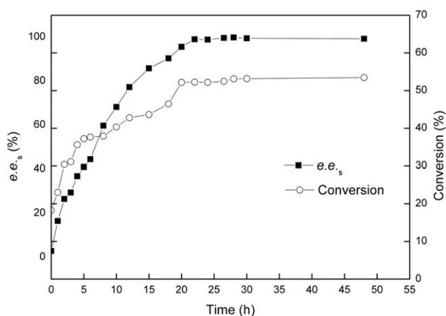
**FIGURE 4** The time course for the enantioselective amidation of (R,S)-1. The reactions were carried out at 40°C and 200 rpm and entailed the use of 100  $\mu$ L (R,S)-1 (0.7 mmol), 200  $\mu$ L methyl 2-tetrahydrofuroate (1.7 mmol), 10 mL MTBE, and 20 mg Novozym 435
