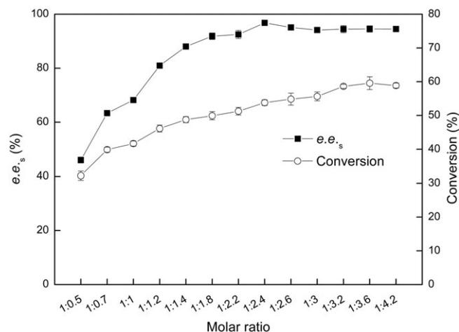
**FIGURE 2** The effects of molar ratios of substrate to acyl donor on the enantioselective amidation of (R,S)-1. The reactions were carried out at 30°C, 200 rpm for 24 hours, and employed 100  $\mu$ L (R,S)-1 (0.7 mmol), different amounts of methyl 2-tetrahydrofuroate, 10 mL MTBE, and 20 mg Novozym 435
