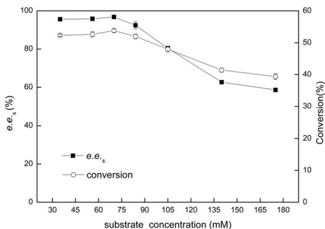
**FIGURE 1** The effects of substrate concentrations on the enantioselective amidation of (R,S)-1. The reactions were carried out at 30°C, 200 rpm for 24 hours, and utilized different concentrations of (R,S)-1, 200 μL methyl 2-tetrahydrofuroate, 10 mL MTBE, and 20 mg Novozym 435
