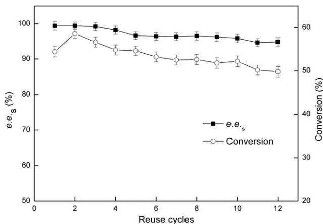
**FIGURE 5** The reuse cycles of immobilized Novozym 435 on the preparation of (S)-1. The reactions were carried out at 40°C at 200 rpm for 22 hours, and entailed 100  $\mu$ L (R,S)-1 (0.7 mmol), 200  $\mu$ L methyl 2-tetrahydrofuroate (1.7 mmol), 10 mL MTBE, and 20 mg Novozym 435
