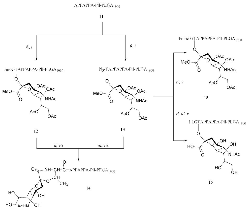
**Scheme 2** Reagents: *i*, TBTU, NEM, DMF; *ii*, 20% piperidine–DMF; *iii*, DTT, DBU, DMF; *iv*, TMSCl, NaI, CH<sub>3</sub>CN; *v*, Fmoc-Aa-OPfp, Dhbt-OH, DMF; *vi*, LiOH, CaCl<sub>2</sub>, 70% Pr<sup>t</sup>OH–H<sub>2</sub>O; *vii*, 80% aqueous hydrazine in MeOH.
