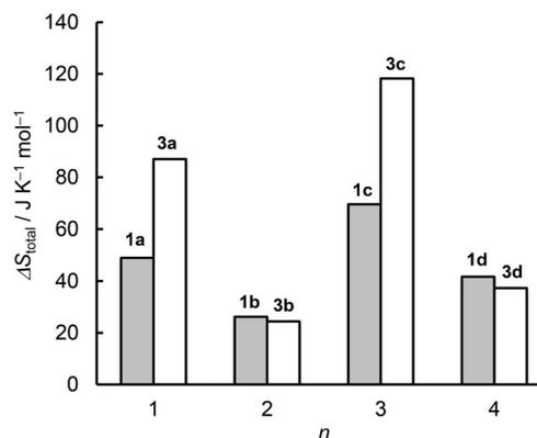
Figure 3. Total phase change entropies  $\Delta S_{\text{total}}$  of **1a–d** and **3a–d** plotted against the carbon number  $n$  in the anion ( $(C_nF_{2n+1}SO_2)_2N$ ).
