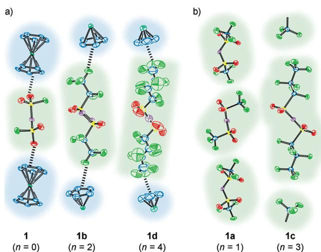
Figure 5. The molecular arrangements around the anions in the columnar structures in the a) mixed-column salts (**1**, **1b**, and **1d**) and b) segregated-column salts (**1a** and **1c**). The molecular structure of **1d** in phase II and those of the other compounds in phase I are shown. Dashed lines indicate cation–anion contacts.
