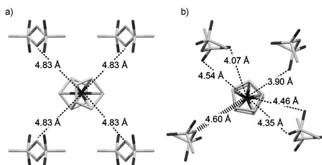
Figure 6. Molecular arrangements around the cation of **1** in a) phase II and b) phase I. Dotted lines show Co...X (X=O, N) distances shorter than 5 Å. The Co...N ion-pair-like interaction in b) is indicated by a thicker dotted line.
