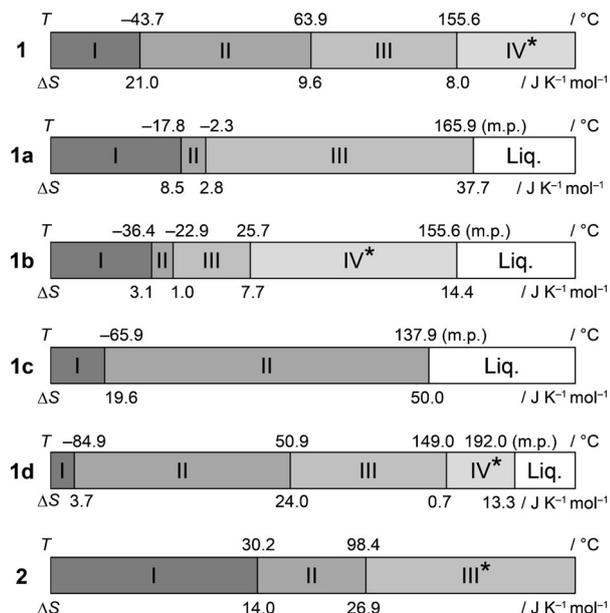
Figure 2. Phase sequences of **1**, **1a–d**, and **2**. The transition temperatures [°C] and transition entropies [J K<sup>–1</sup> mol<sup>–1</sup>] are shown. Highly disordered phases are indicated by an asterisk.
