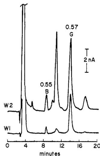
Figure 5. Peak purity assessment of tetrahydropterins in urine by parallel dual-electrode detection: W1 = +300 mV, W2 = +500 mV. The current ratios are listed above their corresponding peaks. Peak identity is the same as those in Figure 2.
