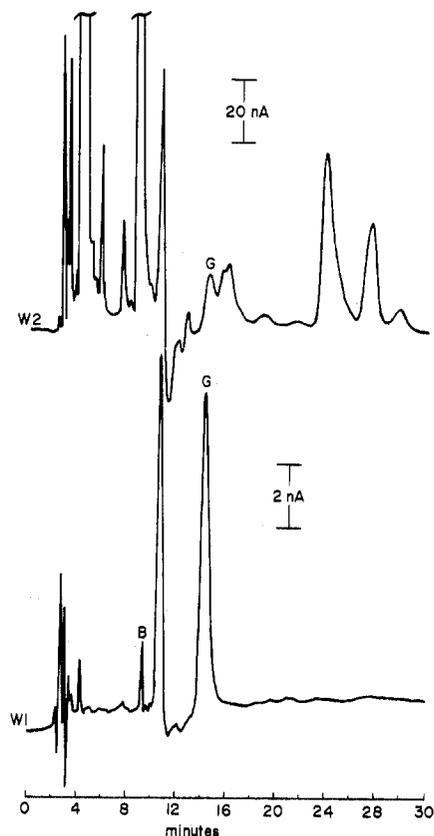
Figure 6. Improved detection of easily oxidized pterins in urine by dual potential monitoring: W1 = +800 mV, W2 = +400 mV. Peak identities are the same as those in Figure 2.
