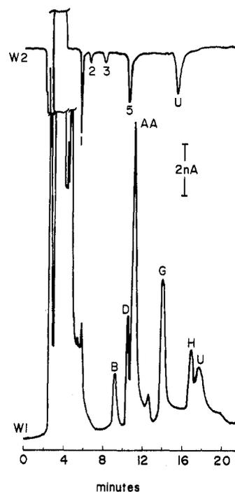
Figure 4. Dual-electrode detection of reduced and oxidized pterins in urine: W1 = +800 mV, W2 = -700 mV. Peak identities are the same as those in Figure 2 except AA is ascorbic acid and U indicates an unidentified peak.
