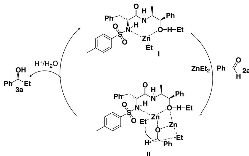
Figure 2. The proposed catalytic cycle.
