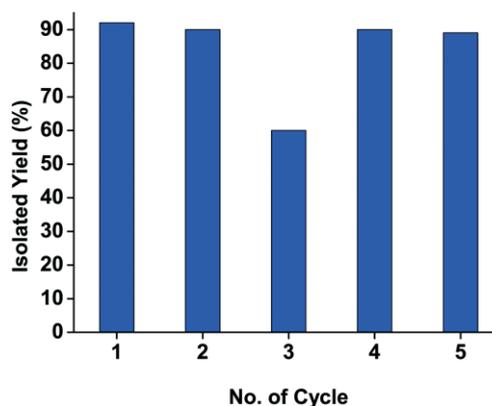
Figure 3. Recyclability chart (recyclability of the oxidant system was tested on the reaction with **1a** and **2a**).
