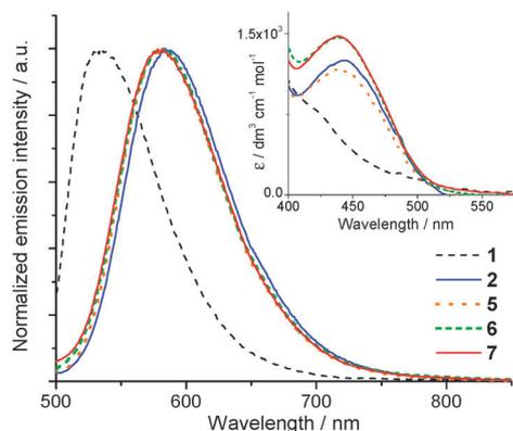
Fig. 1 Normalized emission spectra (inset: low-energy UV-vis absorption bands) of selected complexes ( $10^{-5}$  M; spectra of **3** and **4** closely matches **5–7** and are omitted for clarity) in  $\text{CH}_3\text{CN}$  at 298 K.
