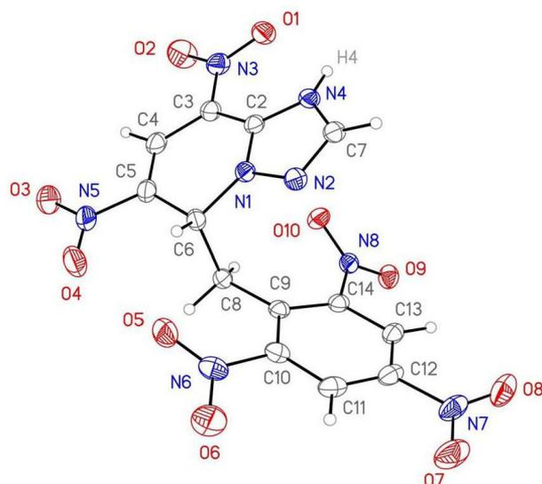
**Figure 2.** Molecular structure of compound **17c** with atoms represented as thermal vibration ellipsoids of 50% probability.
