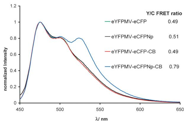
**Fig. 1** Fluorescence spectra of normal enhanced fluorescent protein pairs, normalized at the CFP emission maximum and FRET ratio  $I(527 \text{ nm})/I(475 \text{ nm})$ . Protein concentration  $1 \mu\text{M}$  each, CB[8] concentration  $10 \mu\text{M}$ .
