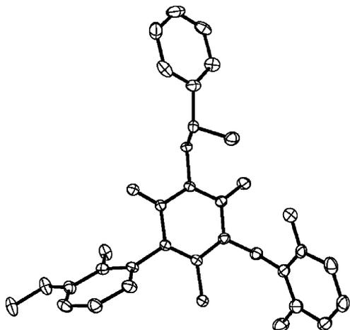
**Figure 2.** X-ray crystal structure of *R*-13b indicates an orthogonal relationship between the 5-(2-fluoro-3-methoxyphenyl) group and the uracil ring.
