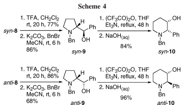
((CF<sub>3</sub>CO)<sub>2</sub>O, THF, Et<sub>3</sub>N, reflux, 48 h and then base-mediated ester hydrolysis) were successful with both *syn*- and *anti*-**9** giving piperidines *syn*-**10** (84% yield) and *anti*-**10** (96% yield) respectively (Scheme 4). The high yield obtained for both of these reactions is notable since it has previously been reported that the *N*-Me version of *syn*-**9** did not undergo the ring expansion.<sup>9b</sup>
